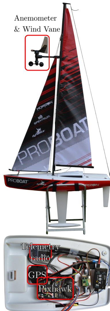
Figure 3: Autonomous sailboat modified for this project (top) and electronics mounted under hatch (bottom).
